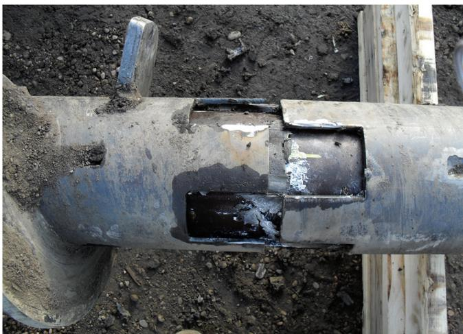
**Figure 1 Two Piece Pile**
