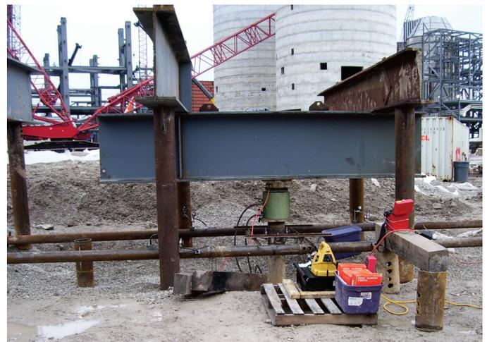
**Figure 3 Traditional Top Down Load Test**
