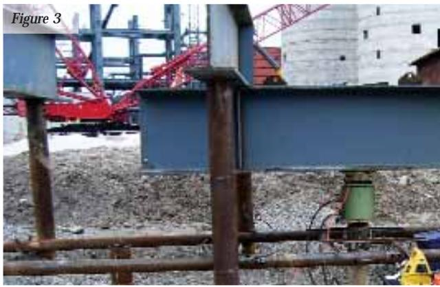
The Osterberg cell (O-Cell) bi-directional testing method enabled relatively low-cost, high-capacity static load testing of bored piles that were otherwise prohibitively expensive or technically impractical. The genius behind the innovation is a specially designed hydraulic jack (O-cell assembly) cast directly into the pile at a predetermined location (Figure 4). After curing or
