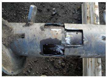
Figure 1 Two Piece Pile
