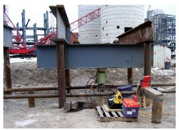
Figure 3 Traditional Top Down Load Test
