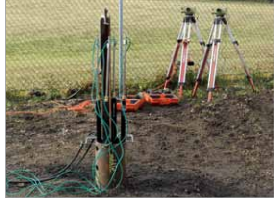
The Osterberg Cell (O-Cell) bi-directional load test.
