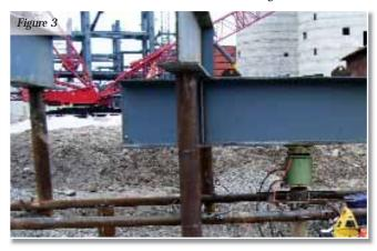
The Osterberg cell (O-Cell) bi-directional testing method enabled relatively low-cost, high-capacity static load testing of bored piles that were otherwise prohibitively expensive or technically impractical. The genius behind the innovation is a specially designed hydraulic jack (O-cell assembly) cast directly into the pile at a predetermined location (Figure 4). After curing or
