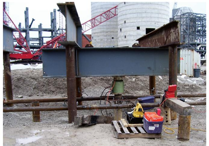
**Figure 3 Traditional Top Down Load Test**
